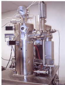
second-generation Nion corrector retrofit to a VG HB 501
