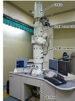
JEOL Delta on a 60 kV microscope
